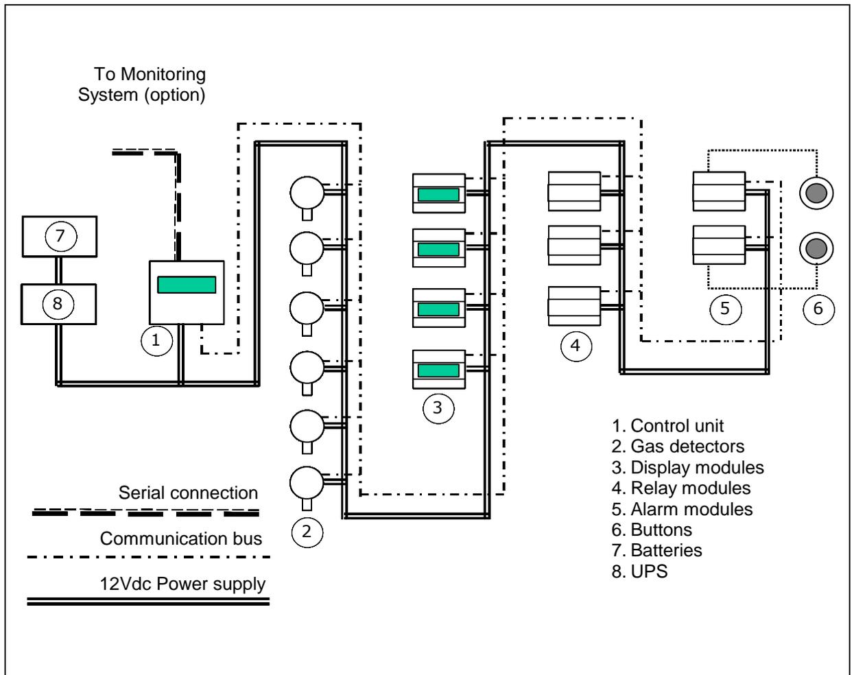
Fig. 2.1 – Layout of the EW40 system
