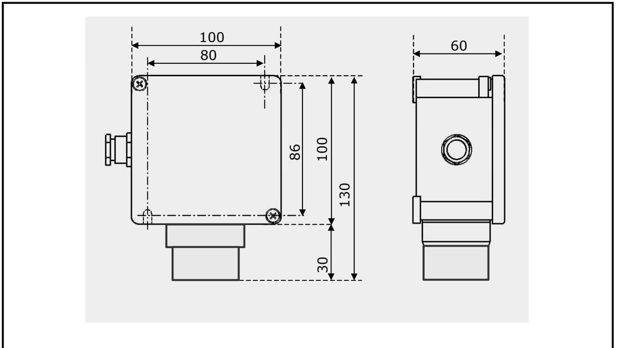
Fig. 12.5 – Dimensions of UR.40.L detectors
