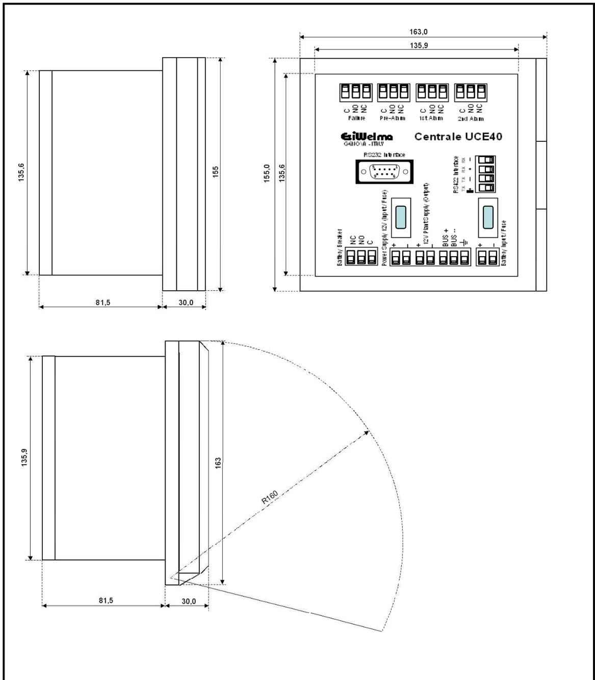
Fig. 12.1 – Dimensions of UCE40... control unit
