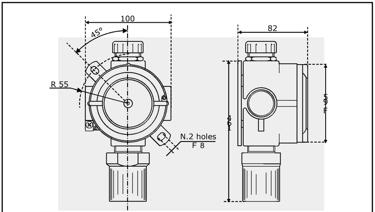
Fig. 12.3 – Dimensions of detectors UR.40.E, UR.40.I
