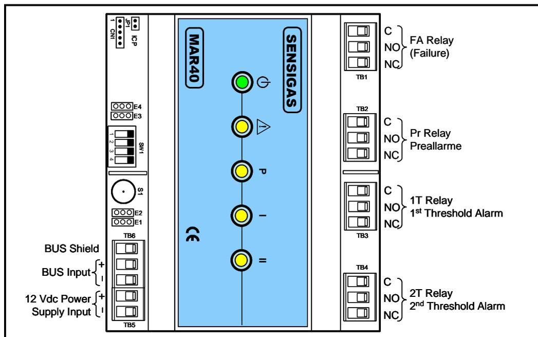
Fig. 4.8 – Terminal boards of the relay module MAR40
