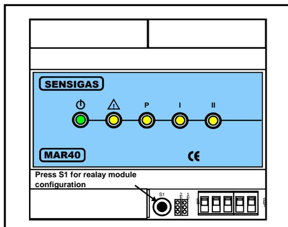
Fig. 6.9 – Configuration of the relay modules
