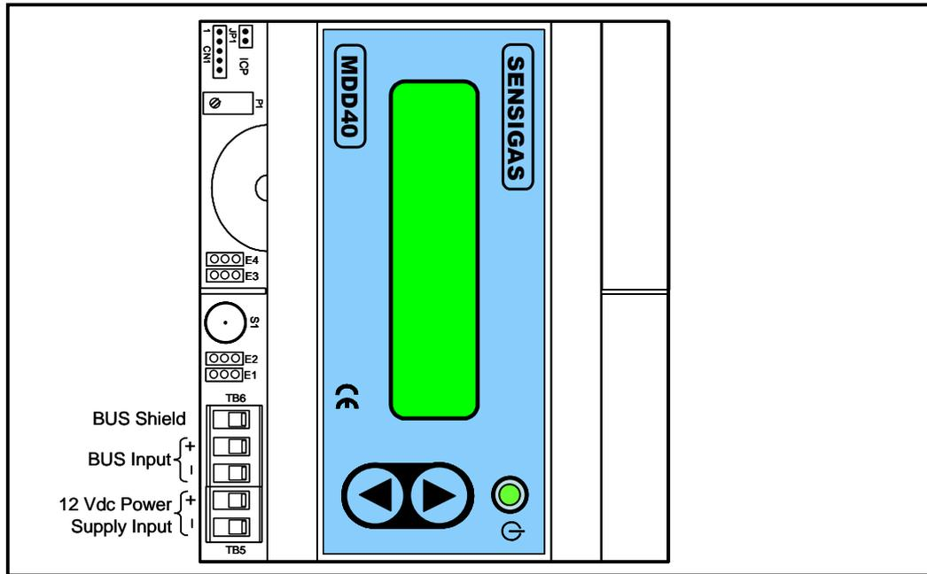
Fig. 4.7 – Terminal board of the display module MDD40
