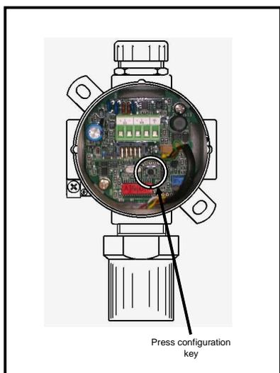
Fig. 6.6 – Configuration of the gas detectors
