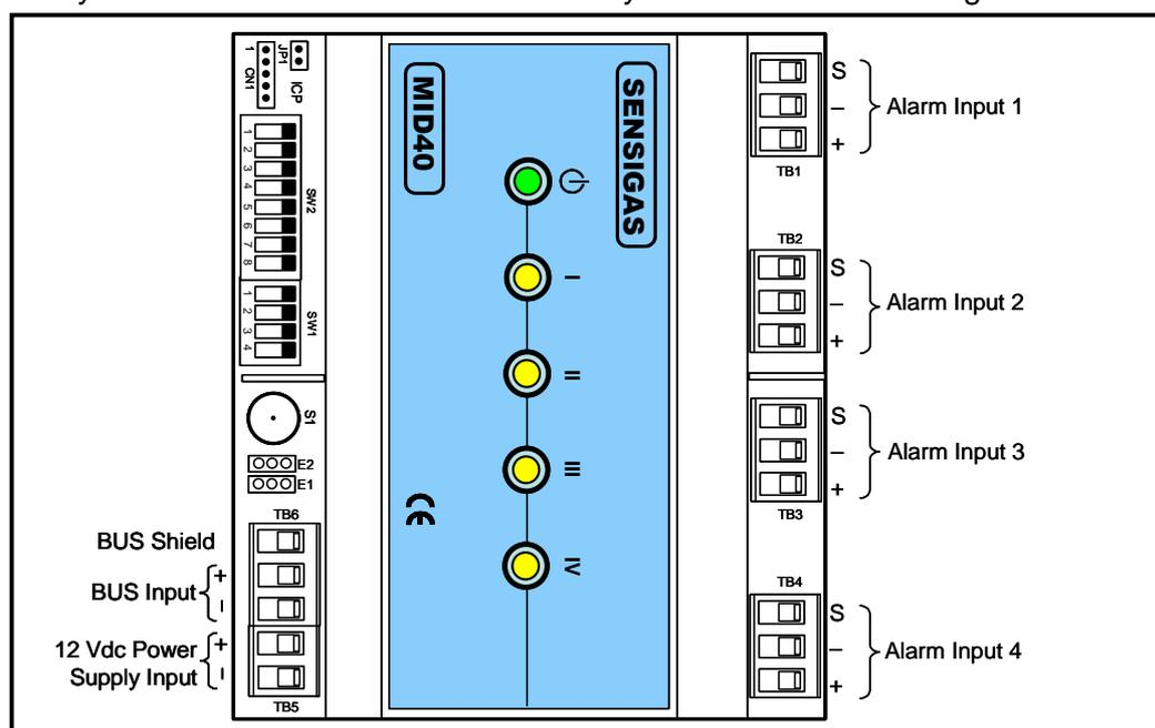
Fig. 4.9 – Terminal board of the alarm module MID40
