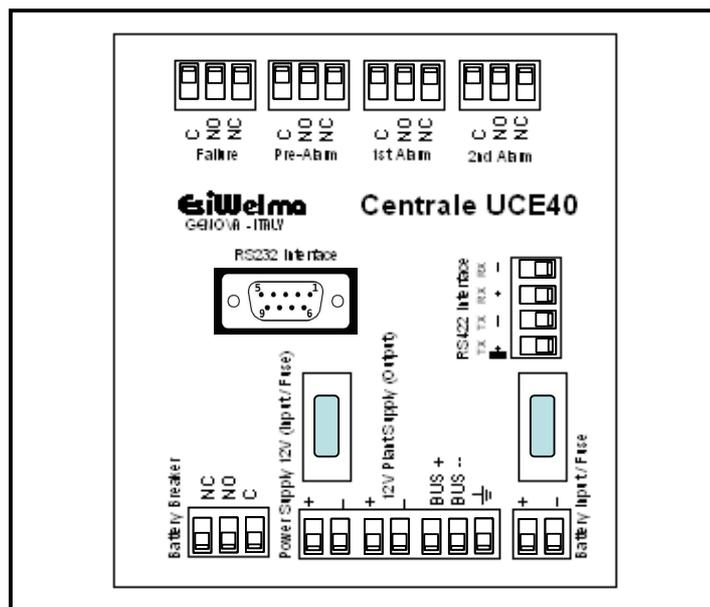
Fig. 4.5 – Terminal board on the control unit UCE40...
