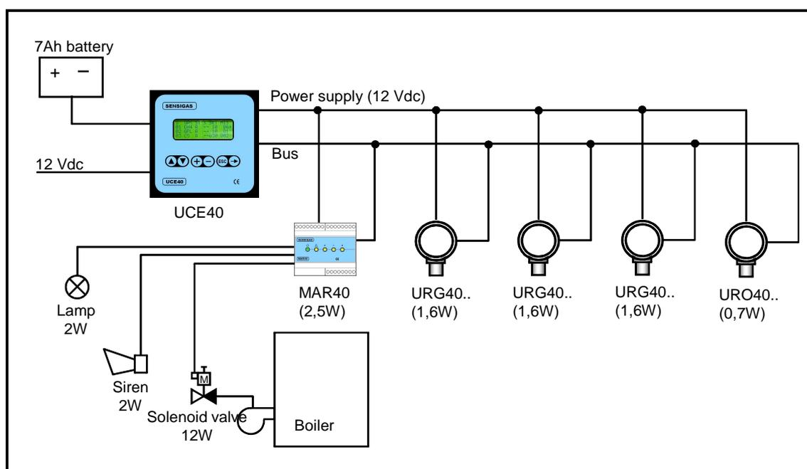
Fig. 4.10 – Basic structure of the system (example)
