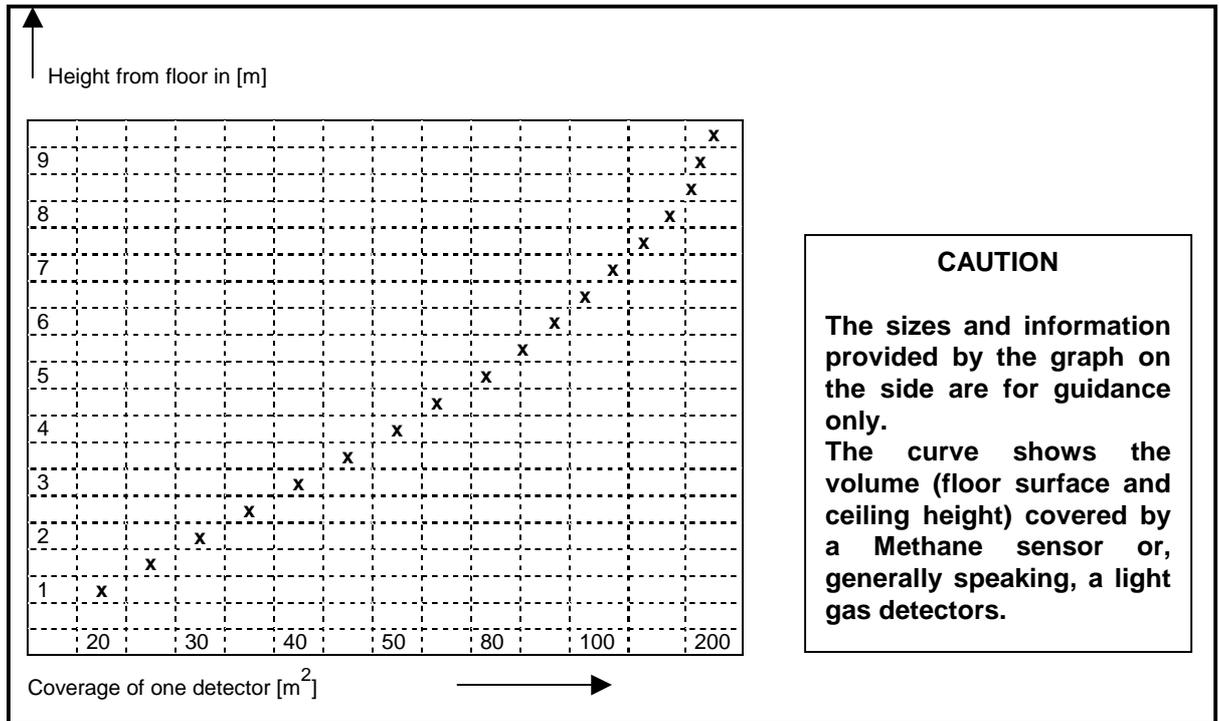
Fig. 3.9 – Coverage of sensors [m<sup>2</sup>]
