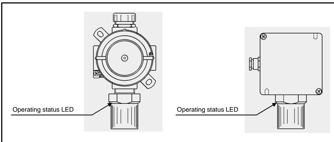
Fig. 6.2 – Function of the LEDs on the UR.40.. sensors
