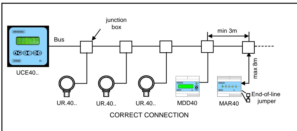
Fig. 4.1 – Example of correct connection
