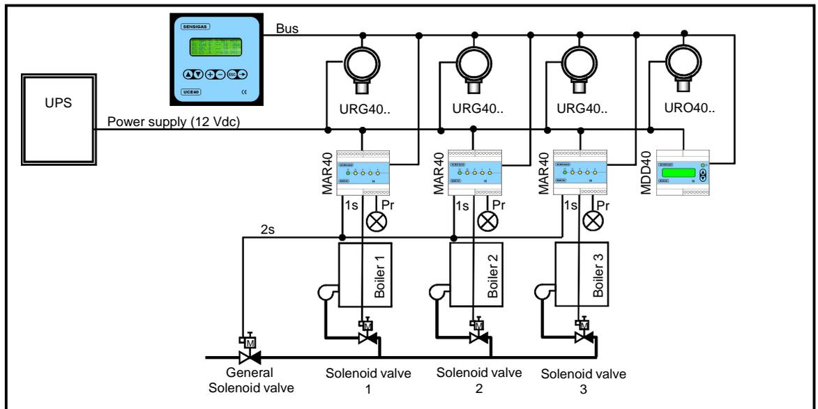
Fig. 4.11 – Extended structure of the system (example)
