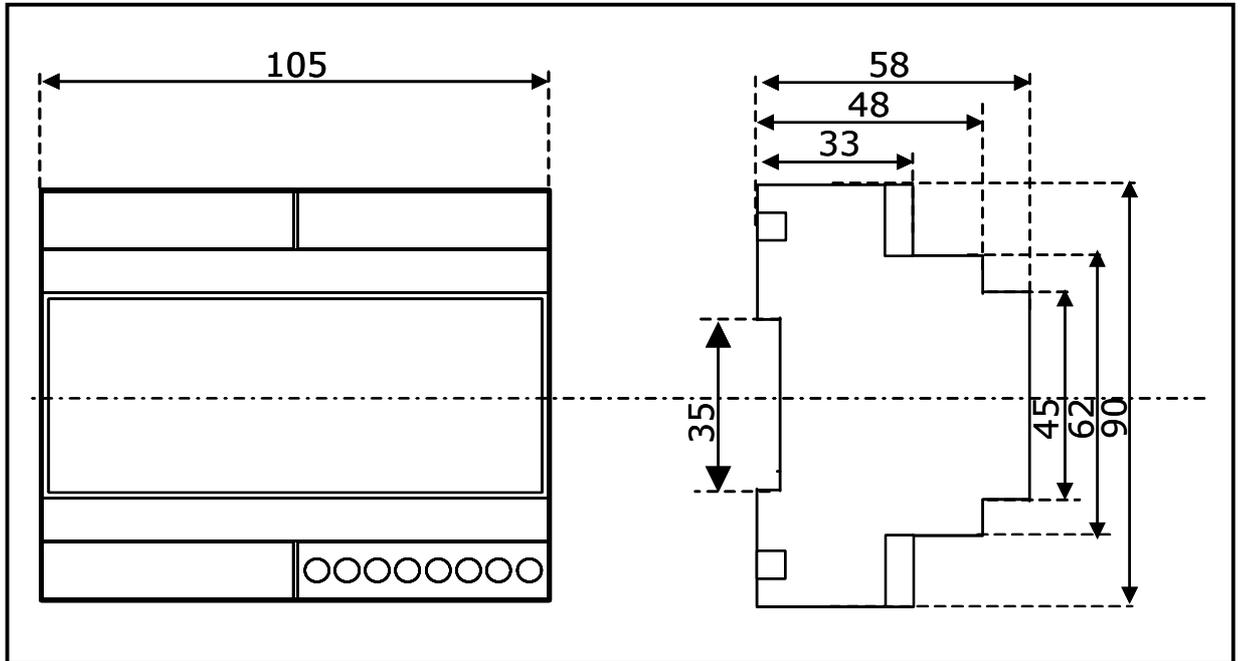
Fig. 12.2 – Dimensions of MAR40, MDD40 and MID40 modules
