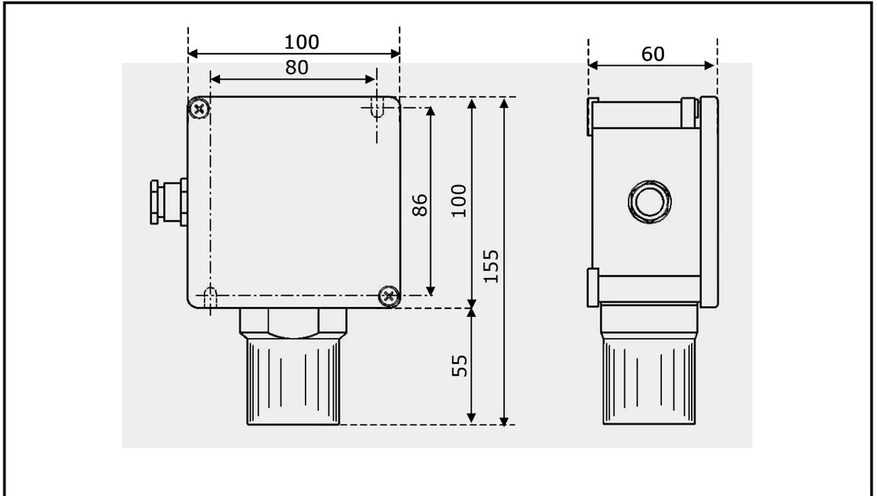
Fig. 12.4 – Dimensions of UR.40.S detectors
